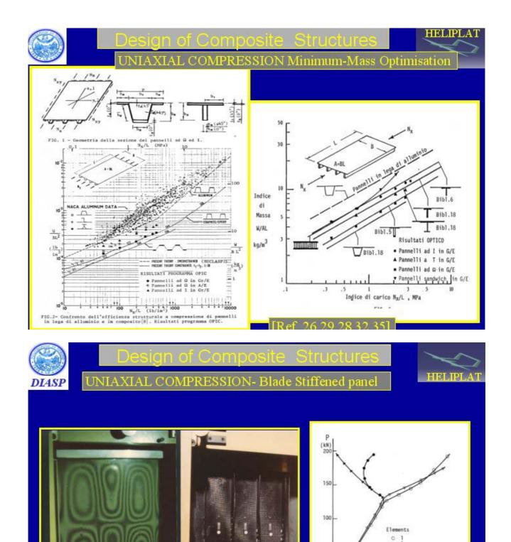
An analytical solution has been developed in order to investigate post-buckling behavior of simply supported and/or fully clamped anisotropic plates under combined biaxial compression and shear load. Since panels are often not perfectly manufactured, initial imperfections are also included in the analysis. Such imperfections in fact considerably influence the out-of-plane displacement behavior of the panel and cannot be ignored. The classical laminate theory has to be modified for
